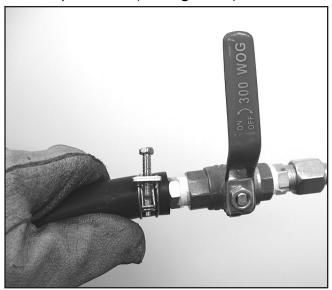
Figure 11. Blast nozzle valve, closed.
